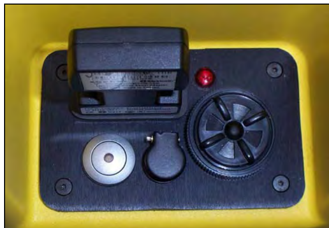
Figure 14. Bluetooth Cordless Serial Adapter Installed in the Gauge
